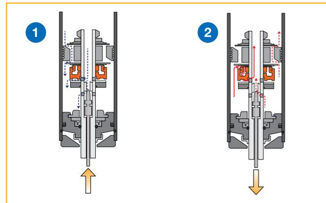
**FIGURE 1:** (Compression flow) At low shaft speeds, oil flows mostly through the shaft jet bleed (lower dotted arrow). At high shaft speeds, oil flows mostly through the compression ports in the piston (upper dotted arrow). At intermediate shaft speeds, which are very critical for comfort, or during sudden shaft accelerations, oil can also escape through the compression ports in the DFV (solid arrow), increasing comfort.
