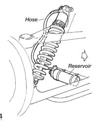
Fit the rubber mounts and the reservoir to the inside tube of the lower triangle link. Use the hose clamps provided to fix the reservoir.
