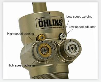
Zeroing adjusters ensures accurate matching between dampers while maintaining reference clicks.
